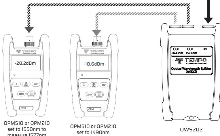
**One power meter can be used to make both measurements.**
